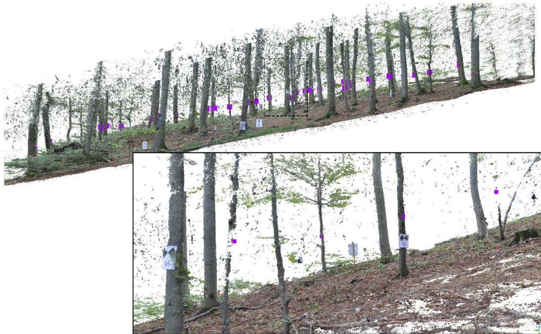
Figure 6. Coloured SfM point cloud of plot 2 in Austria, overlaid with the location of the trees measured by the total station (the magenta square dots). The dashed line indicates the location of the enlarged point cloud at the bottom.
